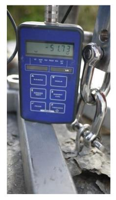
An interesting observation was that the anchors were still holding only a little less than their peak loads when half to two thirds of their length had been extracted. In comparisons between the RAWL R-KER and the Allgrip KMR-RES the inclusion of styrene in the formulation means failure loads are 10kN higher with the Allgrip KMR-RES resin.
