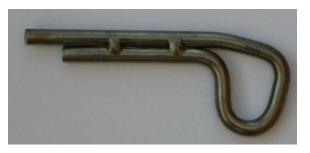
anchor Batch 2". As will be observed later in the report, four out of a sample of sixty four Batch 2 Peco anchors suffered catastrophic metallurgical failure below the 25kN threshold.
